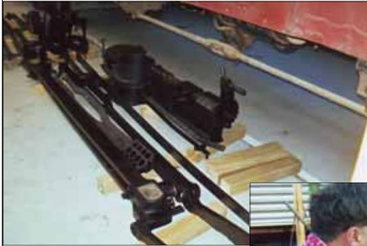
(Lt.) Some of Ralph Boessel's reconditioning work on 1308's reversing gear etc
