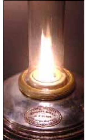
**(Above & below) Two types of colza oil burners. The wick appears to have a solid core and requires a glass chimney to burn properly.**
