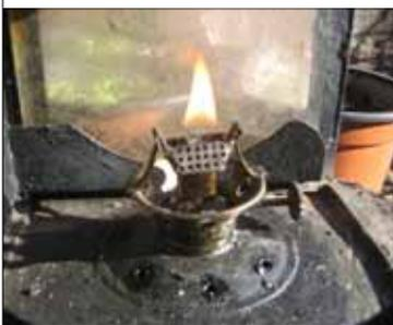
**A kero burner assembly from a signal lamp. Was this type of burner Thornley’s improvement?**
