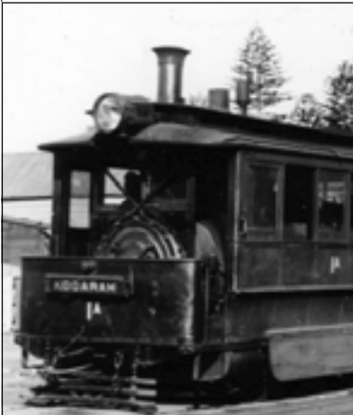
Taken in 1937, this photo shows IA's apron without "cut-outs". It must have been replaced at some time. The foot-plate continues to appear "straight".
