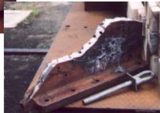
The broken corner of the cylinder, prepared for welding to cylinder, already welded together from two pieces.
