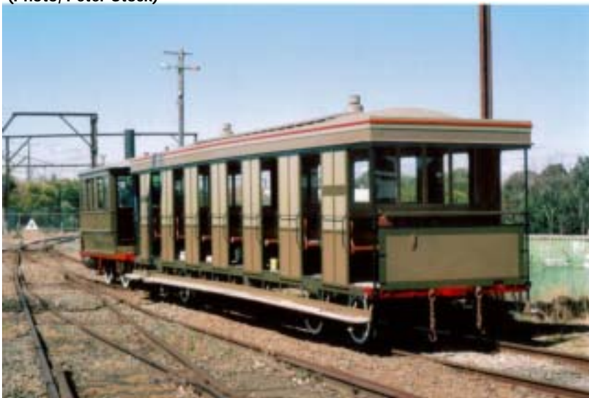
The trailer car looks resplendent as the tram heads out towards the outer end of the compound. Handbrakes have since been installed and footboards painted. Doors are still to be fitted. (Photo, Peter Stock)
