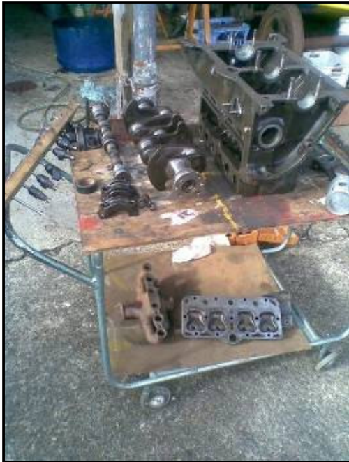
Above: The motor of the Prefect truck dismantled, mid way through its mechanical overhaul. Photo: Bruce Coxon
