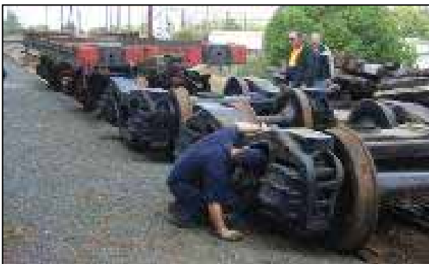
Above: Tender bogies and Tender frame (sitting on temporary bogies) just after arrival at Valley Heights. Photo: Col Burne.
