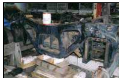
Left: The bogie frame lifted and wheel sets free to allow work to commence. Photo: Andrew Tester.
